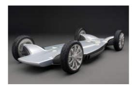
An all-electric system would easily fit into the Skateboard. This would free an automobile manufacturer to create any body design.
